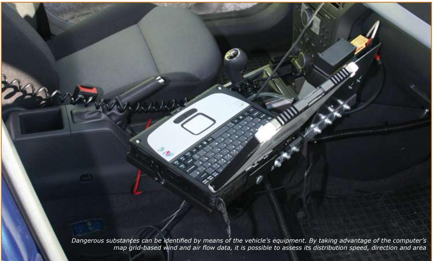
*Dangerous substances can be identified by means of the vehicle's equipment. By taking advantage of the computer's map grid-based wind and air flow data, it is possible to assess its distribution speed, direction and area*
